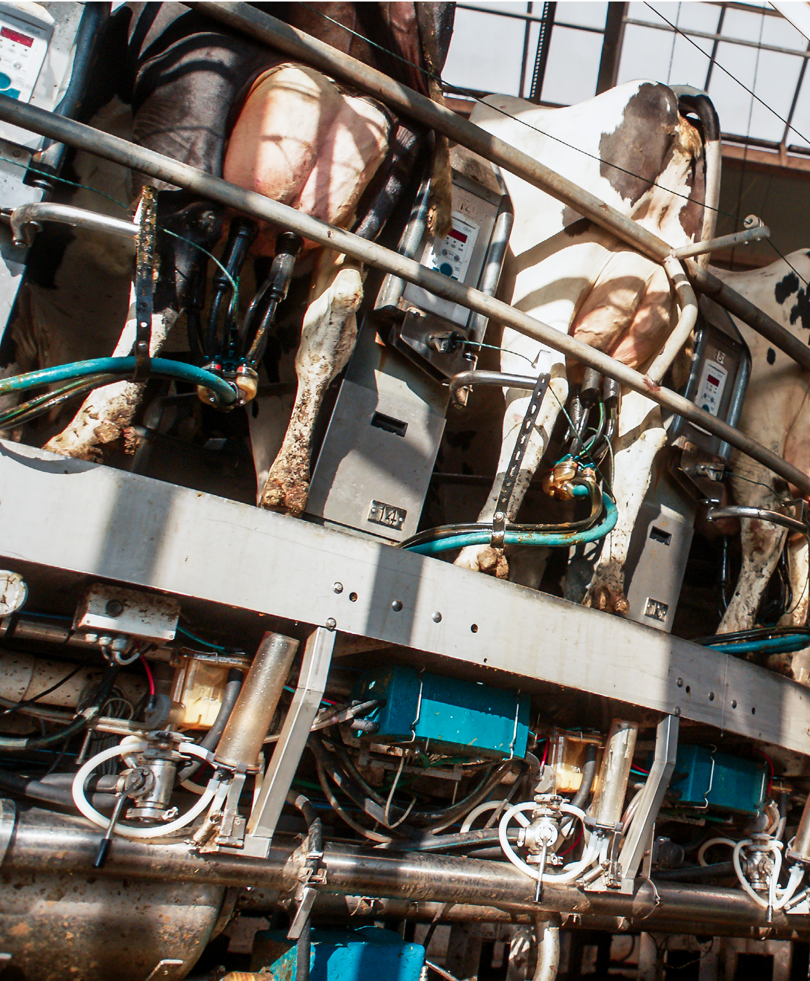
The circular milking barn at the Dairy Campus in Leeuwarden, Netherlands, where cows move through an automated carousel that exemplifies the spatial logics of high-efficiency milk production
