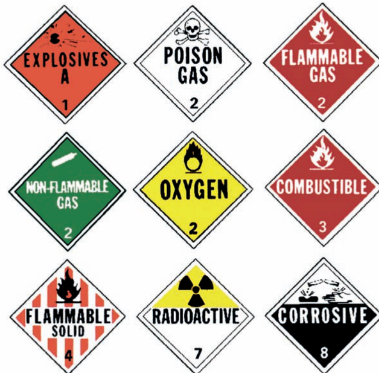
Figure 1-1 Warning placards indicating presence of hazardous material.
