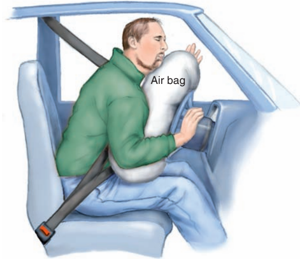
Air bag and three-point restraint prevents collisions 2 and 3.
