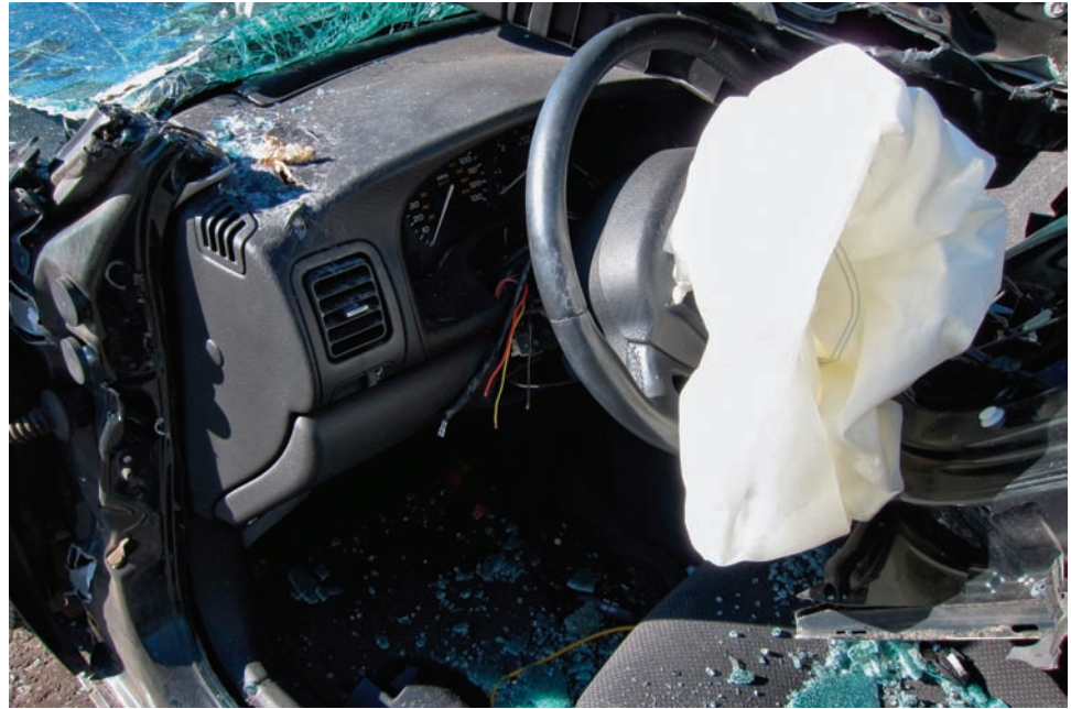
Figure 1-3 Lift the collapsed air bag to note whether or not there is a deformity of the steering wheel. (Olivier Le Queinec/Shutterstock)
