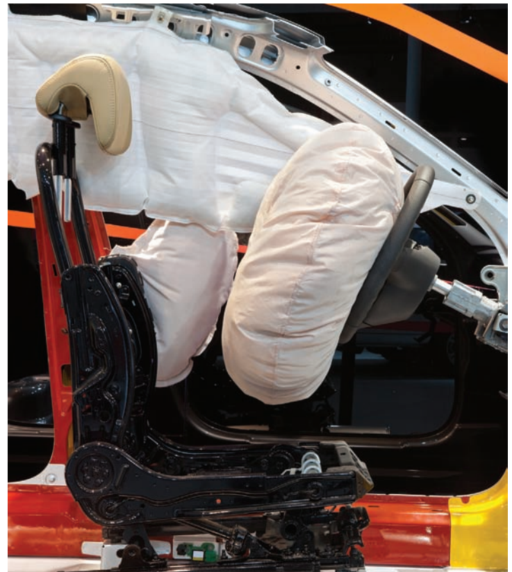
Figure 1-6 Side airbags and air curtains can pose a hazard to responders if the devices did not activate in the collision. Note: See the Access: First on Scene—Rapid Vehicle Entry Provider Manual from ITLS for more information about rendering nondeployed airbags safe. (testing/Shutterstock)
