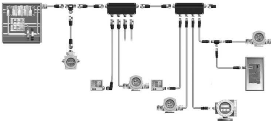
Figure 1.25 – Topologie d'un bus Fieldbus Foundation.
